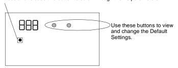
There are 15 total programmable parameters for the Display. If no RP03 remote probe is used, the Display will default with 12 parameters. If remote probe is selected the other three parameters will be viewable (\*).
