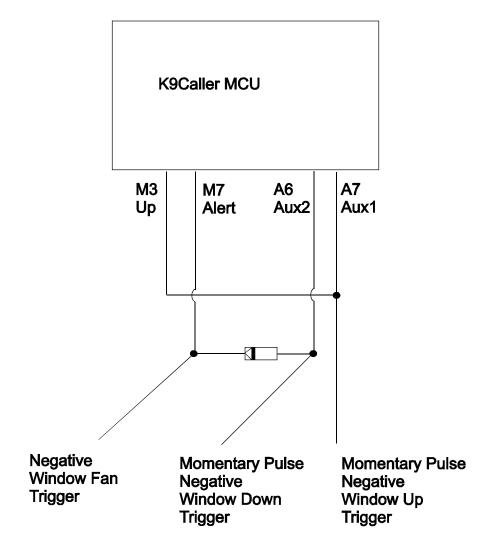
Use Aux1 for remote window roll up and Aux 2 for window roll down
